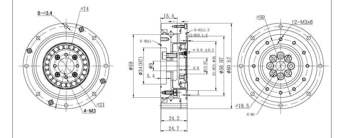
L2/D1: Please don't interfere the minimum safety dimension when assembling with circular spline.
